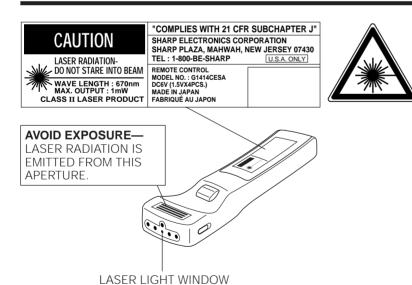
The laser pointer on the remote control emits a laser beam from the laser light window shown in the figure to the left. The laser emitted is a class II laser; therefore, do not look into the laser window or shine the laser beam on yourself or other people. The three marks to the left are the caution labels for the laser beam.
